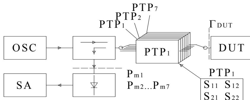
**Fig. 1. Measurement system with 7-state perturbation two-port.**
